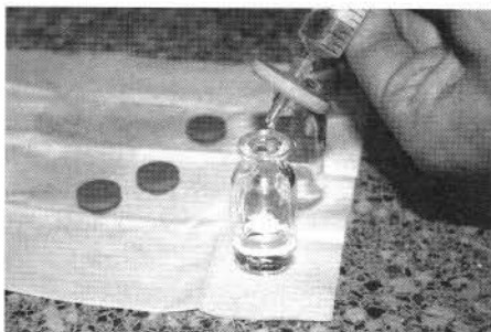
Syringe filtration of steroid solution. Use of new (sterile) vial reduces chance of recontamination.
